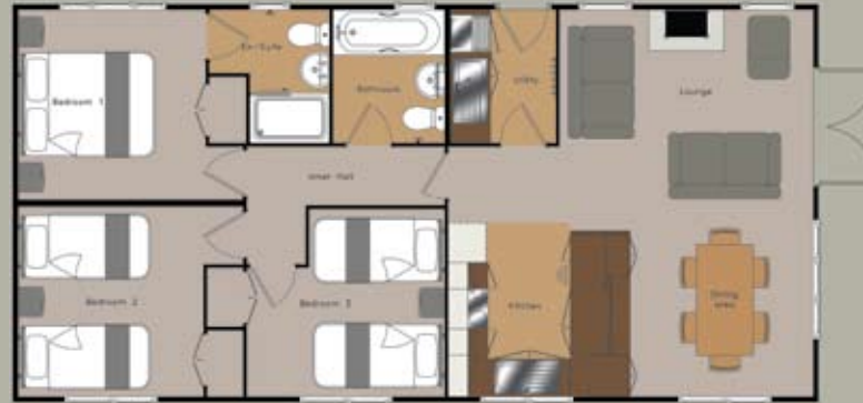
Overall size: 40 x 20ft. 3 Bed en-suite with utility Gross Floor Area: 790sqft (73.44sqm)
