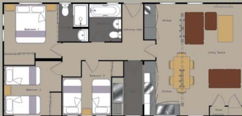
Overall size: 42 x 20ft. 3 Bed en-suite with utility Gross Floor Area: 830sqft (77.12sqm)
