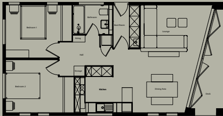
Overall size: 42 x 22ft 2 Bed. Shower over bath Gross Internal Area: 835sqft (77.59sq/m)
